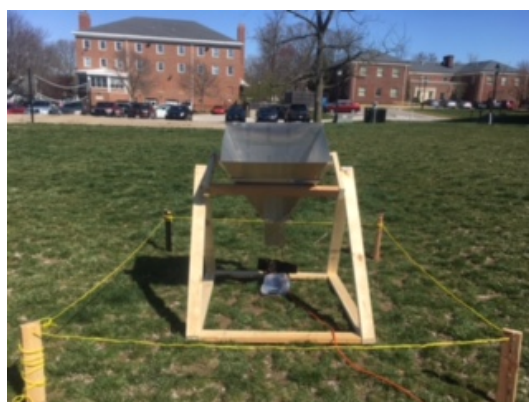
The radio telescope built in AdLab by Hamza Moudou (‘21) and used by Elijah Scurlock (‘23) to detect the Milky Way.
